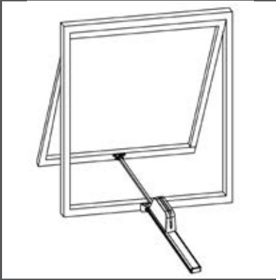
Installation on top hinged window
