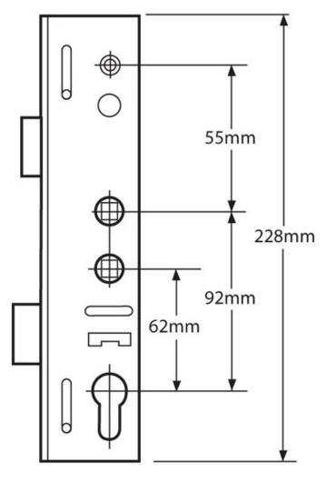
Lockmaster gearbox centre case 35mm - 62mm / 92mm Centre Case Gearbox can be used to replace a like for like Centre Case when it is no longer working. In addition, the Lockmaster gearbox 35mm - 62mm / 92mm double spindle version can be installed as an upgrade to your existing product if only a single spindle to allow a different handle operation if desired
