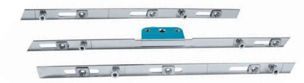
This espag rod is extremely versatile, it is available with a 13mm or 16mm wide inline 1 metre strip with 4 mushrooms however each side can be cropped up to 4 times in 10cm increments. The centre case has an 8mm follower, 2 threaded holes and slides 20mm to the side which rotates the follower from square to diamond.
