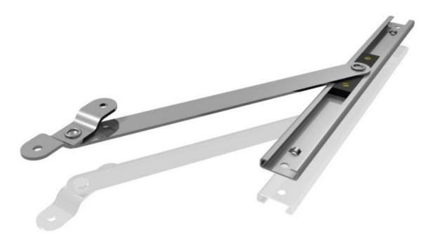
On side hung windows supported by standard butt hinges (and in some cases friction stays) the friction arm offers distinct advantages over the conventional peg stay. It is totally concealed when the vent is closed and offers no internal obstruction when opened.
